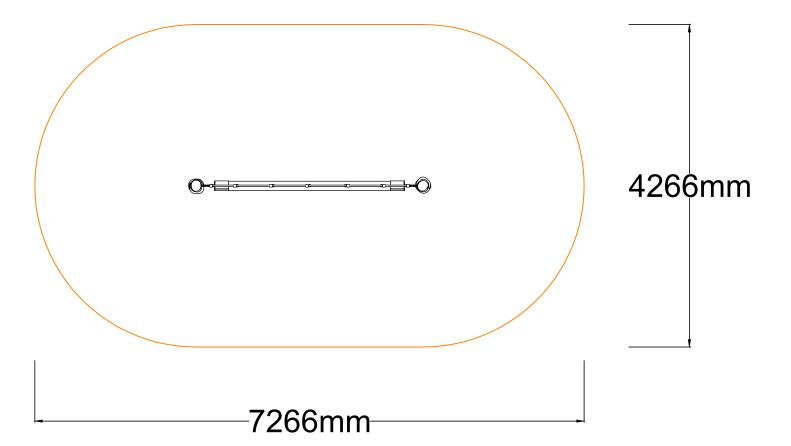
The min. recommended fall zone around the entire play structure is shown. This zone is to be free of all tripping or collision hazards (ie. roots, rocks, border material, etc).
