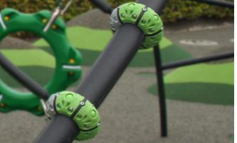
Modular connectors eliminate the need for welding during assembly. Root disc is made using aluminum injection technique and has 6 connection points. Used connection points are also made using the aluminum injection technique and non-used connection points are covered with PA6
