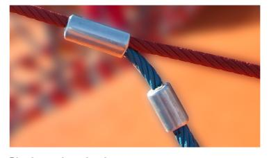
Single-casing aluminum cast connectors are compressed with 300 tons to avoid moving and premature wear. "E (end stop) connector" is shapely and pleasant to grip with no sharp angles or edges. These connectors are fastened to main frame either to welded flanges on main frame or with "C" aluminum clamps to main frame.
