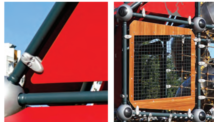
High quality panels made of HPL panels are milled to provide a smooth, gently rounded edge. The thickness of the panels varies according to its purpose for floors, roofs, and walls. These panels are connected to steel pipes or profiles with cast aluminum panel clamps or flanges. To increase the visibility of interior of the equipment, some panels are equipped with 5 mm thick anti-climb steel meshes. This wire mesh is placed within either steel or HPL frame.
