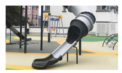
UV resistant with high value of light fastness rotomolded polyethylene parts are used to form the structure. All parts are manufactured with double wall technique with the thickness between 4-6 mm.
