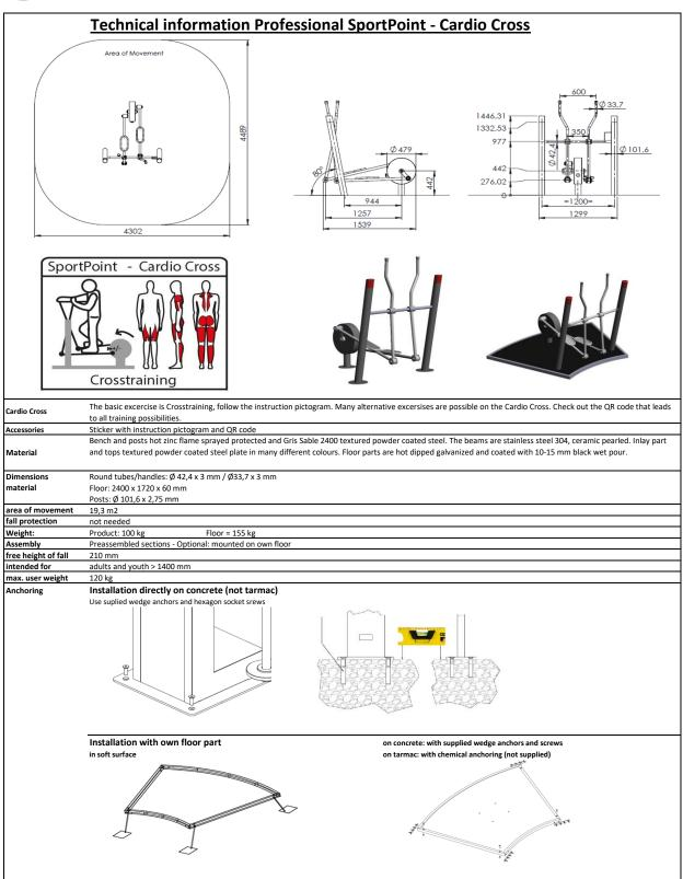
When 3 or more floors are connected no anchoring into the ground is needed EN16630:2015 - for permanently installed outdoor fitness equipment Certification:
