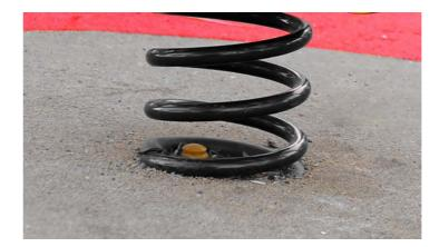
Spring cross-section diameter is 22 mm, spring diameter 200 mm, and height 400 mm with a maximum of 8 helical turns is one of the best spring manufactured for playgrounds and carries the brand of Eibach ™ The product will be manufactured from " cold drawn spring " DH -EN 10270-1 high carbon spring steel.
