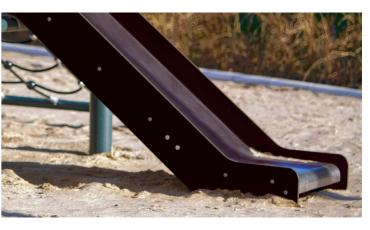
This slide type is very resistant to wear and tear remaining in mint condition for years. Stainless steel material is 2 mm thick. Approved product according to EN 1176 norms. Sides of the slide is HPL or HDPE with rounded edges.
