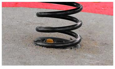
Spring cross-section diameter is 22 mm, spring diameter 200 mm, and height 400 mm with a maximum of 8 helical turns is one of the best spring manufactured for playgrounds and carries the brand of Eibach  $^{\text{\tiny M}}$  The product will be manufactured from " cold drawn spring " DH -EN 10270-1 high carbon spring steel.
