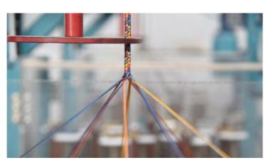
CmrRope ™ is formed by 6 strands of galvanized wires and a core either steel or fiber. Each strand is tightly braided with Polyester which is adhered to galvanized wires with a patented method to create a solid surface where polyester meets with wires. So extra protection is achieved against friction and vandalism. Surface is extremely abrasion and UV resistant also fire retardant.
