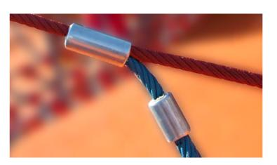
Single-casing aluminum cast connectors are compressed with 300 tons to avoid moving and premature wear. "E (end stop) connector" is shapely and pleasant to grip with no sharp angles or edges. These connectors are fastened to main frame either to welded flanges on main frame or with "C" aluminum clamps to main frame.
