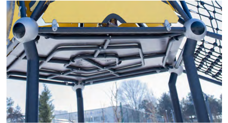
Metal parts are comprised of ST 37 Steel with a 3-step metal finish. Sandblasting and solvent-free zinc primer coating and electrostatic powder paint application is inherently corrosion resistant under extreme weather conditions and UV.
