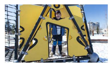
High quality panels made of HPL panels are milled to provide a smooth, gently rounded edge. The thickness of the panels varies according to its purpose for floors, roofs, and walls. These panels are connected to steel pipes or profiles with cast aluminum panel clamps or flanges.
