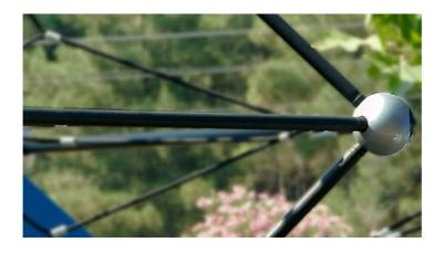
Metal parts are comprised of ST 37 Steel with a 3-step metal finish. Sandblasting and solvent-free zinc primer coating and electrostatic powder paint application is inherently corrosion resistant under extreme weather conditions and UV.
