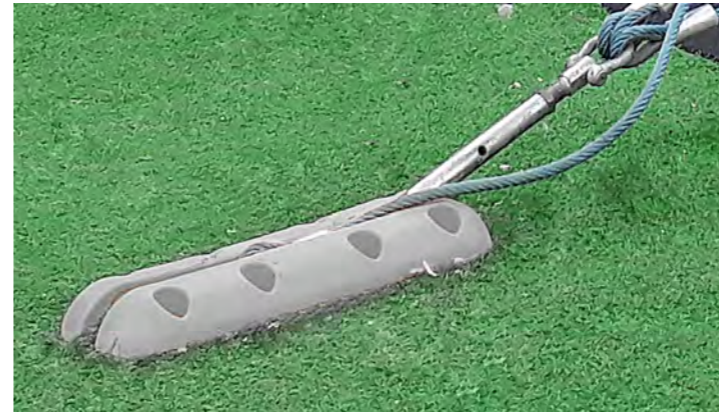
Sandblasted – solvent free zinc primer treated, and powder coated ST 37 metal anchor contains multiple connection points to allow adjusting and connection of the safety rope. For main mast, a cocoon shall be placed in the center. This two parts assembly allows less pressure to cocoon edges and easier installation. Corner anchors are covered with rotomolded polyethylene covers.
