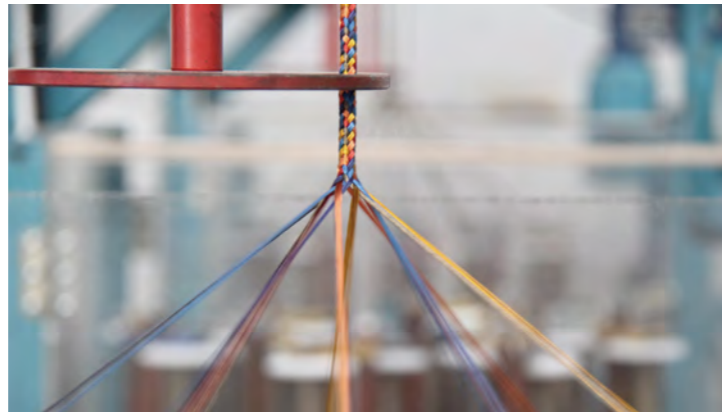
CmrRope™ is formed by 6 strands of galvanized wires and a core either steel or fiber. Each strand is tightly braided with Polyester which is adhered to galvanized wires with a patented method to create a solid surface where polyester meets with wires. So extra protection is achieved against friction and vandalism. Surface is extremely abrasion and UV resistant also fire retardant.
