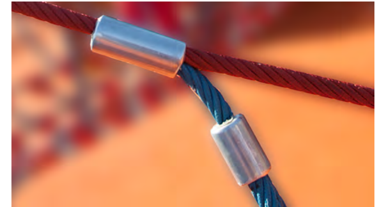
Single-casing aluminum cast connectors are compressed with 300 tons to avoid moving and premature wear. “E (end stop) connector” is shapely and pleasant to grip with no sharp angles or edges. These connectors are fastened to main frame either to welded flanges on main frame or with “C” aluminum clamps to main frame.
